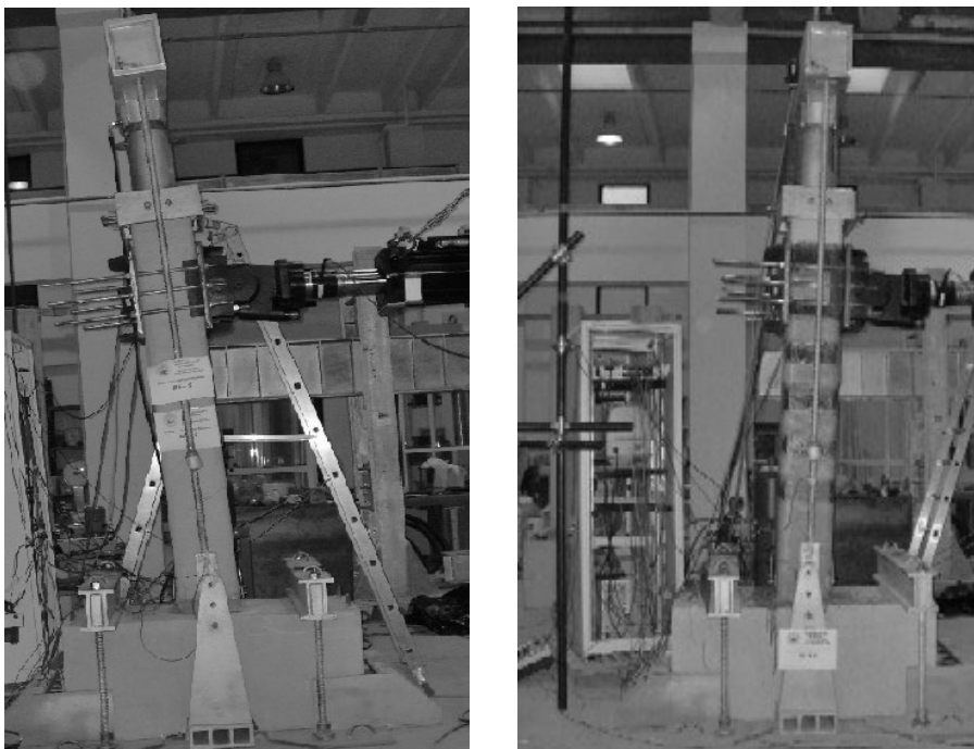
Fig. 5. Unconfined “C3-S” column (left) and GFRP confined “C4-S-G” column (right) during the test.
